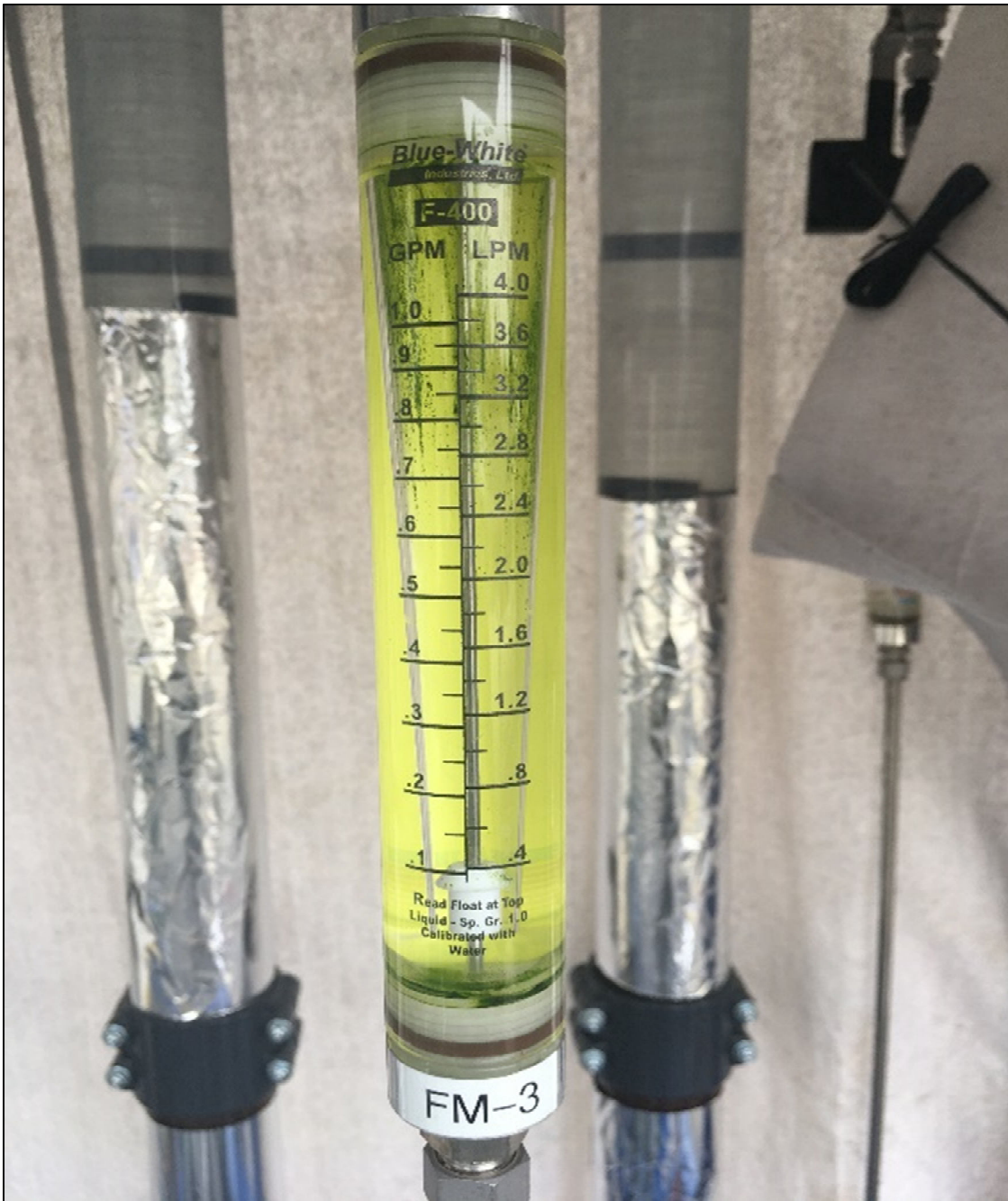
June 16, 2020, Algae is observed for the first time in a flowmeter, belonging to AV1240PFAS GAC.
