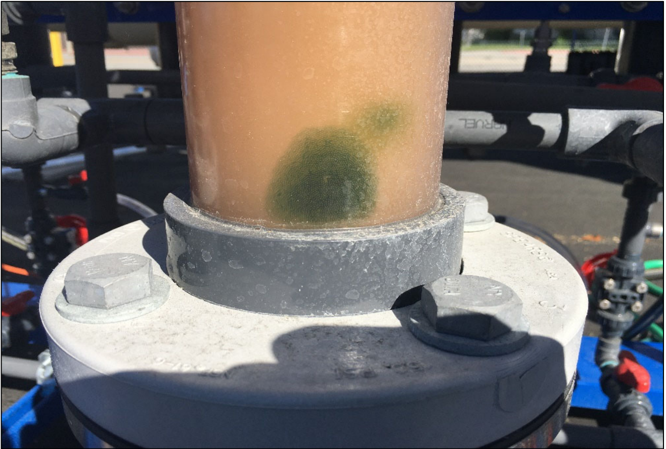
June 9, 2020, Algae is observed for the first time in the PFA694E column.
